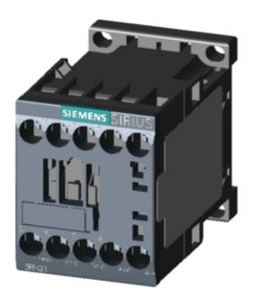
COUPLING CONTACTOR RELAY, 3NO+1NC, DC 24V, 0.85..1.85\*US, W/ INTEGRATED DIODE, SIZE S00, SCREW TERMINAL
