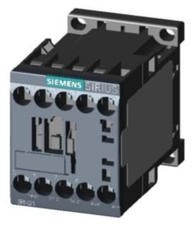
COUPLING CONTACTOR RELAY, 3NO+1NC, DC 24V, 0.7...1.25\*US, W/ INTEGRATED SUPPRESSOR DIODE, SIZE S00, SCREW TERMINAL
