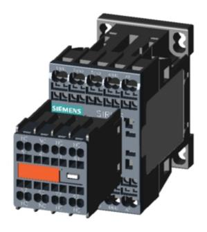
CONTACTOR RELAY, 4NO+4NC, AC 230V, 50/60 HZ, SZ S00, SPRING-LOADED TERMINAL, PERMANENT AUX. SWITCH, FOR SUVA APPLICATIONS
