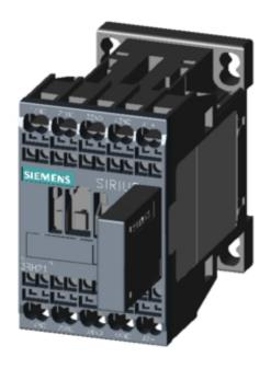
COUPLING CONTACTOR RELAY, 3NO+1NC, DC 24V, 0.85..1.85\*US, W/ PLUGGED-ON VARISTOR, SZ S00, SPRING-LOADED TERMINAL
