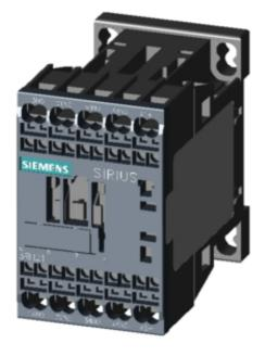
COUPLING CONTACTOR RELAY, 3NO+1NC, DC 110V, 0.7..1.25\*US, W/ INTEGRATED SUPPRESSOR DIODE, SZ S00, SPRING-LOADED TERMINAL
