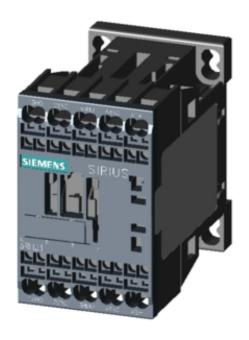
CONTACTOR RELAY, 3NO+1NC, DC 125V, SZ S00, SPRING-LOADED TERMINAL
