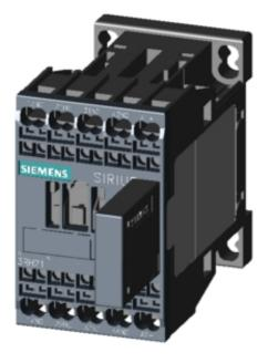
COUPLING CONTACTOR RELAY, 2NO+2NC, DC 24V, 0.85..1.85\*US, W/ PLUGGED-ON VARISTOR, SZ S00, SPRING-LOADED TERMINAL
