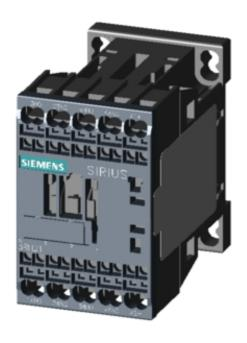
COUPLING CONTACTOR RELAY, 4NO, DC 24V, 0.7...1.25\*US, W/ INTEGRATED DIODE, SZ S00, SPRING-LOADED TERMINAL
