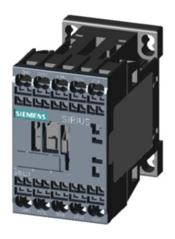
COUPLING CONTACTOR RELAY, 2NO+2NC, DC 24V, 0.85..1.85\*US, W/ INTEGRATED DIODE, SZ S00, SPRING-LOADED TERMINAL
