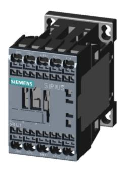
COUPLING CONTACTOR RELAY, 3NO+1NC, DC 24V, 0.85..1.85\*US, W/ INTEGRATED DIODE, SZ S00, SPRING-LOADED TERMINAL
