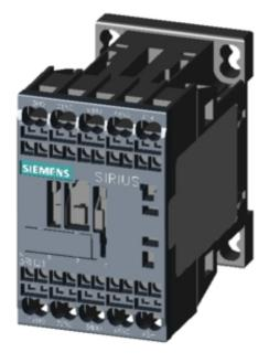
COUPLING CONTACTOR RELAY, 3NO+1NC, DC 24V, 0.7...1.25\*US, W/ INTEGRATED SUPPRESSOR DIODE, SZ S00, SPRING-LOADED TERMINAL
