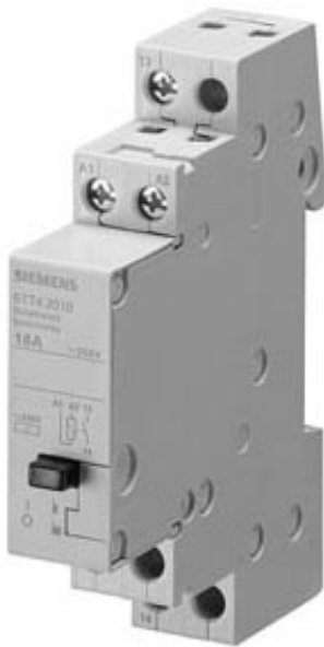
RELAY, N-TYPE WITH 4 NO CONTACT FOR AC 230V 16A CONTROL AC 8V
