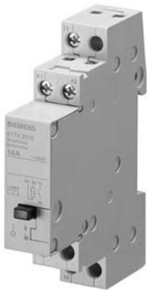
RELAY, N-TYPE WITH 2 NO CONTACT FOR AC 230V 16A CONTROL AC 24V
