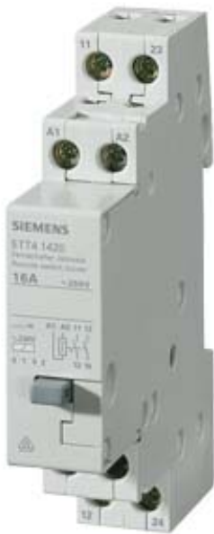
REMOTE SWITCH WITH 2 NO WITH JALOUSIE CONTROL CONTACT FOR AC 230, 400V 16A CONTROL AC 12V
