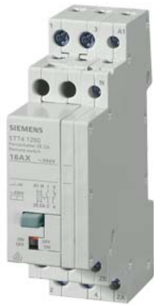
REMOTE SWITCH WITH 1 NO AND 1 NC WITH CENTRAL ON-OFF-FUNCTION CONTACT FOR AC 230, 400V 16A CONTROL AC 230V
