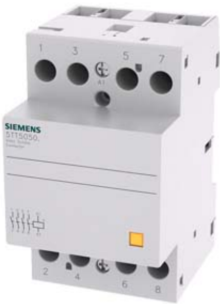
INSTA CONTACTOR WITH 4 NO CONTACTS CONTACT FOR AC 230, 400V 63A ACTIVATION ACDC24V
