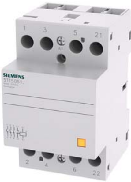
INSTA CONTACTOR WITH 3 NO CONT. AND 1 NC CONT. CONTACT FOR AC 230, 400V 63A ACTIVATION AC230V DC220V
