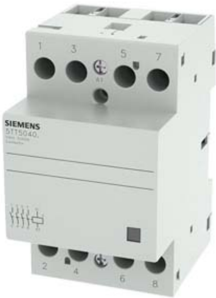
INSTA CONTACTOR WITH 4 NO CONTACTS CONTACT FOR AC 230, 400V 40A ACTIVATION ACDC24V
