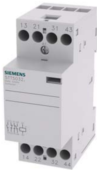
INSTA CONTACTOR WITH 2 NO CONT. AND 2 NC CONT. CONTACT FOR AC 230, 400V 25A ACTIVATION AC230V DC220V
