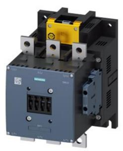
Power contactor, AC-3 265 A, 132 kW / 400 V Coil AC 50/60 Hz and DC 200-277 V x (0.8-1.1) F-PLC input 24 V DC 3-pole size S10 Auxiliary contacts 2 NO + 2 NC Main circuit: Busbar Control and auxiliary circuit: screw terminal
