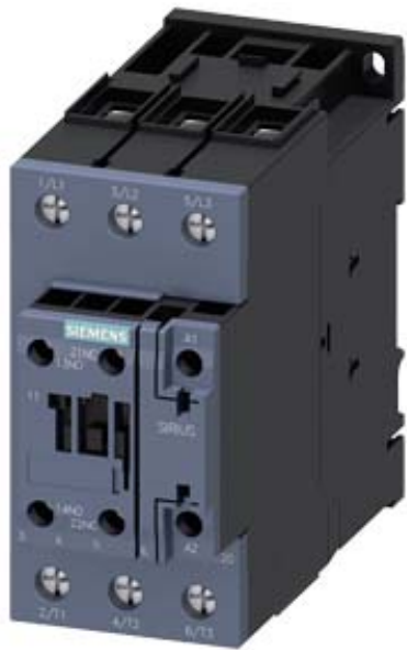
CONTACTOR,AC3:18.5KW/400V, 1NO+1NC, 230V AC 50HZ, 3-POLE, SIZE S2, SCREW TERMINAL
