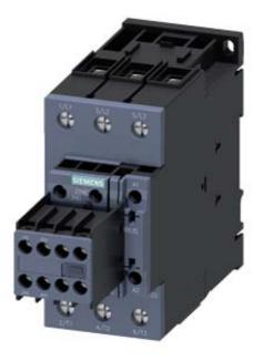
CONTACTOR,AC3:18.5KW/400V, 1NO+1NC,400VAC50HZ/400.440V60HZ 3-POLE, SIZE S2, SCREW TERMINAL
