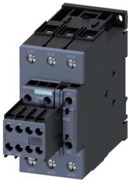
CONTACTOR,AC3:22KW/400V, 1NO+1NC,400VAC50HZ/400.440V60HZ 3-POLE, SIZE S2, SCREW TERMINAL
