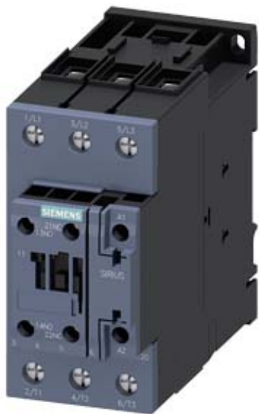
CONTACTOR,AC3:22KW/400V, 1NO+1NC,400VAC50HZ/400.440V60HZ 3-POLE, SIZE S2, SCREW TERMINAL
