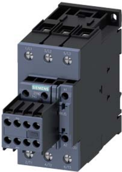
CONTACTOR,AC3:30KW/400V, 2NO+2NC, 230V AC 50/60HZ, 3-POLE, SIZE S2, SCREW TERMINAL
