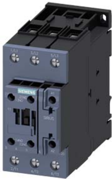
CONTACTOR,AC3:30KW/400V, 1NO+1NC,110VAC 50HZ/120V 60HZ, 3-POLE, SIZE S2, SCREW TERMINAL
