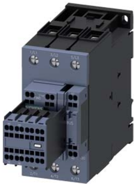
CONTACTOR,AC3:30KW/400V, 2NO+2NC, 110V AC 50HZ, 3-POLE, SIZE S2, SPRING-TYPE TERMINAL
