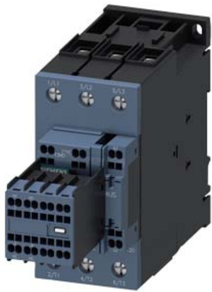
CONTACTOR,AC3:30KW/400V, 2NO+2NC, 48 - 80V AC/DC, WITH VARISTOR, 3-POLE, SIZE S2, SPRING-TYPE TERMINAL
