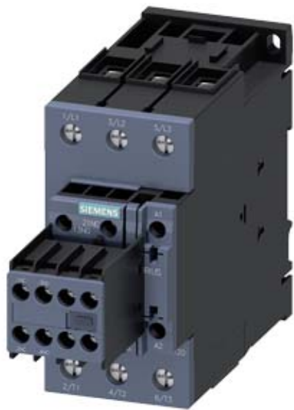
CONTACTOR,AC3:37KW/400V, 2NO+2NC, 230V AC 50/60HZ, 3-POLE, SIZE S2, SCREW TERMINAL
