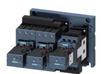
STAR-DELTA (WYE-D.) COMBINATION AC3:22/30KW/400V 110V AC 50/60HZ SIZE S2, SCREW CONNECTION ELECTR. AND MECH. INTERLOCK 3NO+3NC INTEGR.
