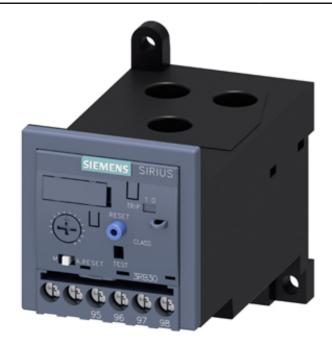
OVERLOAD RELAY 12.5...50 A FOR MOTOR PROTECTION SIZE S2, CLASS 20E STAND-ALONE INSTALLATION MAIN CIRCUIT: STR.-THR. TRANSF. AUX. CIRCUIT: SCREW TERMINAL MANUAL-AUTOMATIC-RESET
