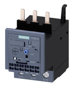
OVERLOAD RELAY 12.5...50 A FOR MOTOR PROTECTION SIZE S2, CLASS 20E FOR MOUNTING ONTO CONTACTORS MAIN CIRCUIT: SCREW TERMINAL AUX. CIRCUIT: SPRING-T. TERM. MANUAL-AUTOMATIC-RESET
