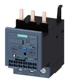
OVERLOAD RELAY 12.5...50 A FOR MOTOR PROTECTION SIZE S2, CLASS 5E...30E FOR MOUNTING ONTO CONTACTORS MAIN CIRCUIT: SCREW TERMINAL AUX. CIRCUIT: SPRING-TYPE TERM. MANUAL-AUTOMATIC-RESET INT. GROUND FAULT DETECTION
