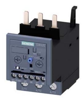
OVERLOAD RELAY 12.5...50 A FOR MOTOR PROTECTION SIZE S2, CLASS 5E...30E FOR MOUNTING ONTO CONTACTORS MAIN CIRCUIT: SCREW TERMINAL AUX. CIRCUIT: SCREW TERMINAL MANUAL-AUTOMATIC-RESET INT. GROUND FAULT DETECTION
