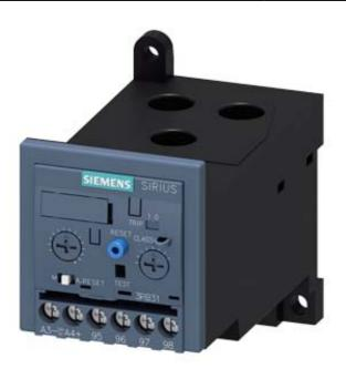
OVERLOAD RELAY 12.5...50 A FOR MOTOR PROTECTION SIZE S2, CLASS 5E...30E STAND-ALONE INSTALLATION MAIN CIRCUIT: STR.-THR. TRANSF. AUX. CIRCUIT: SCREW TERMINAL MANUAL-AUTOMATIC-RESET INT. GROUND FAULT DETECTION
