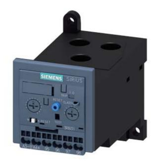
OVERLOAD RELAY 12.5...50 A FOR MOTOR PROTECTION SIZE S2, CLASS 5E...30E STAND-ALONE INSTALLATION MAIN CIRCUIT: STR.-THR. TRANSF. AUX. CIRCUIT: SPRING-TYPE TERM. MANUAL-AUTOMATIC-RESET INT. GROUND FAULT DETECTION
