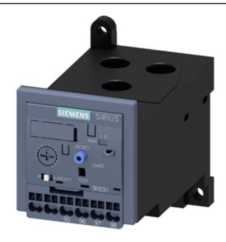
OVERLOAD RELAY 12.5...50 A FOR MOTOR PROTECTION SIZE S2, CLASS 10E STAND-ALONE INSTALLATION MAIN CIRCUIT: STR.-THR. TRANSF. AUX. CIRCUIT: SPRING-T. TERM. MANUAL-AUTOMATIC-RESET
