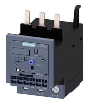
OVERLOAD RELAY 12.5...50 A FOR MOTOR PROTECTION SIZE S2, CLASS 10E FOR MOUNTING ONTO CONTACTORS MAIN CIRCUIT: SCREW TERMINAL AUX. CIRCUIT: SPRING-T. TERM. MANUAL-AUTOMATIC-RESET
