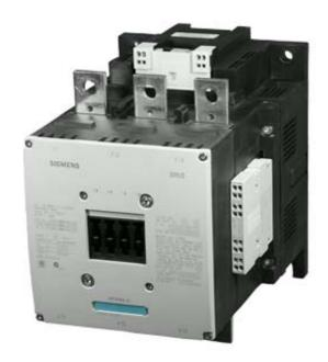
CONTACTOR, 250KW/400V/AC-3 AC(40...60HZ)/DC OPERATION UC 200-277V AUXILIARY CONTACTS 2NO+2NC 3-POLE, SIZE S12 BAR CONNECTIONS ELECTRONIC OPERATING MECHANISM WITH 24 V DC PLC INTERFACE CAGE CLAMP TERMINAL
