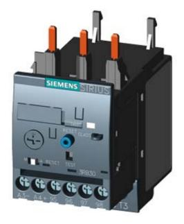
OVERLOAD RELAY 0.1...0.4 A FOR MOTOR PROTECTION SIZE S0, CLASS 20 CONTACTOR ASS. MAIN CIRCUIT: SCREW CONN. AUX.CIRCUIT: SCREW CONN. MANUAL-AUTOM.-RESET
