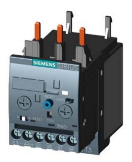
OVERLOAD RELAY 0.32...1.25 A FOR MOTOR PROTECTION SIZE S0, CLASS 5...30 CONTACTOR ASS. MAIN CIRCUIT: SCREW CONN. AUX.CIRCUIT: SCREW CONN. MANUAL-AUTOM.-RESET INT. GROUND FAULT DETECTION
