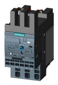
OVERLOAD RELAY 0.32...1.25 A FOR MOTOR PROTECTION SIZE S0, CLASS 5...30 CONTACTOR ASS. MAIN CIRCUIT: SPR.-LOAD.TERM. AUX.CIRCUIT: SPR.-LOAD.TERM. MANUAL-AUTOM.-RESET INT. GROUND FAULT DETECTION
