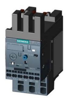
OVERLOAD RELAY 0.32...1.25 A FOR MOTOR PROTECTION SIZE S0, CLASS 20 CONTACTOR ASS. MAIN CIRCUIT: SPR.-LOAD.TERM. AUX.CIRCUIT: SPR.-LOAD.TERM. MANUAL-AUTOM.-RESET
