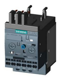
OVERLOAD RELAY 0.1...0.4 A FOR MOTOR PROTECTION SIZE S00, CLASS 5...30 CONTACTOR ASS. MAIN CIRCUIT: SPR.-LOAD.TERM. AUX.CIRCUIT: SPR.-LOAD.TERM. MANUAL-AUTOM.-RESET INT. GROUND FAULT DETECTION
