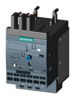
OVERLOAD RELAY 0.32...1.25 A FOR MOTOR PROTECTION SIZE S00, CLASS 20 CONTACTOR ASS. MAIN CIRCUIT: SPR.-LOAD.TERM. AUX.CIRCUIT: SPR.-LOAD.TERM. MANUAL-AUTOM.-RESET
