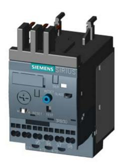
OVERLOAD RELAY 0.32...1.25 A FOR MOTOR PROTECTION SIZE S00, CLASS 10 CONTACTOR ASS. MAIN CIRCUIT: SPR.-LOAD.TERM. AUX.CIRCUIT: SPR.-LOAD.TERM. MANUAL-AUTOM.-RESET
