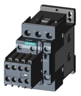
CONTACTOR, AC-3, 11KW/400V, 2NO+2NC, AC 220V 50/60HZ, 3-POLE, SZ S0 SCREW TERMINAL REMOVABLE AUX. SWITCH
