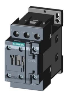
CONTACTOR, AC-3, 11KW/400V, 1NO+1NC, AC 230V 50/60HZ, 3-POLE, SZ SO SCREW TERMINAL
