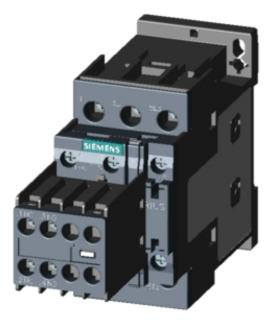
CONTACTOR, AC-3, 11KW/400V, 2NO+2NC, AC110V 50/60HZ, 3-POLE, SZ S0 SCREW TERMINAL REMOVABLE AUX. SWITCH
