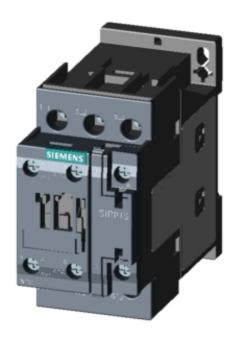
CONTACTOR, AC-3, 11KW/400V, 1NO+1NC, AC110V 50HZ, 3-POLE, SZ SO SCREW TERMINAL
